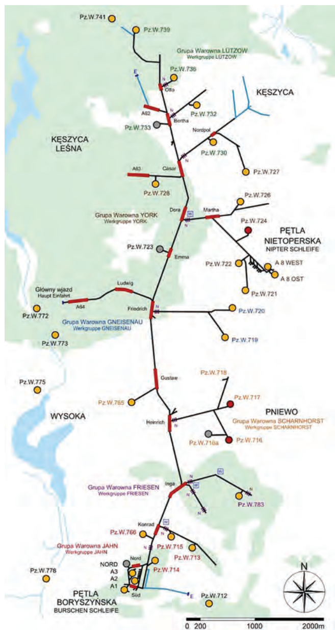
Plan of the underground Miedzyrzecz Rejon Umocniony (MRU) bunker supply system. The 'main line' runs north-south, the rail line has several side branches with the named stations shown in red. On lines without stations there are no rail lines, so the supplies must presumably have been intended to be manhandled on trolleys or similar
